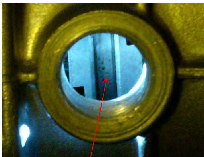
1st & 2nd gear dog, viewed thru oil fill hole in neutral
