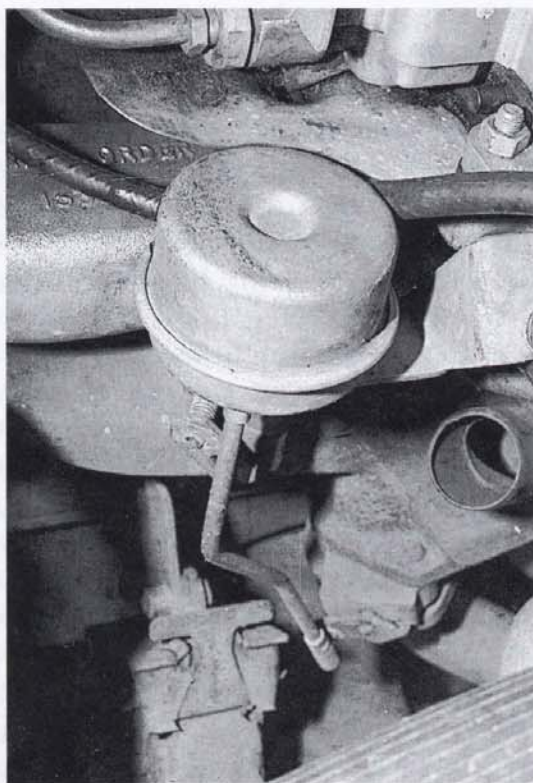
The EFE actuator which operates butterfly valves to divert exhaust flow to heat the inlet manifold.
