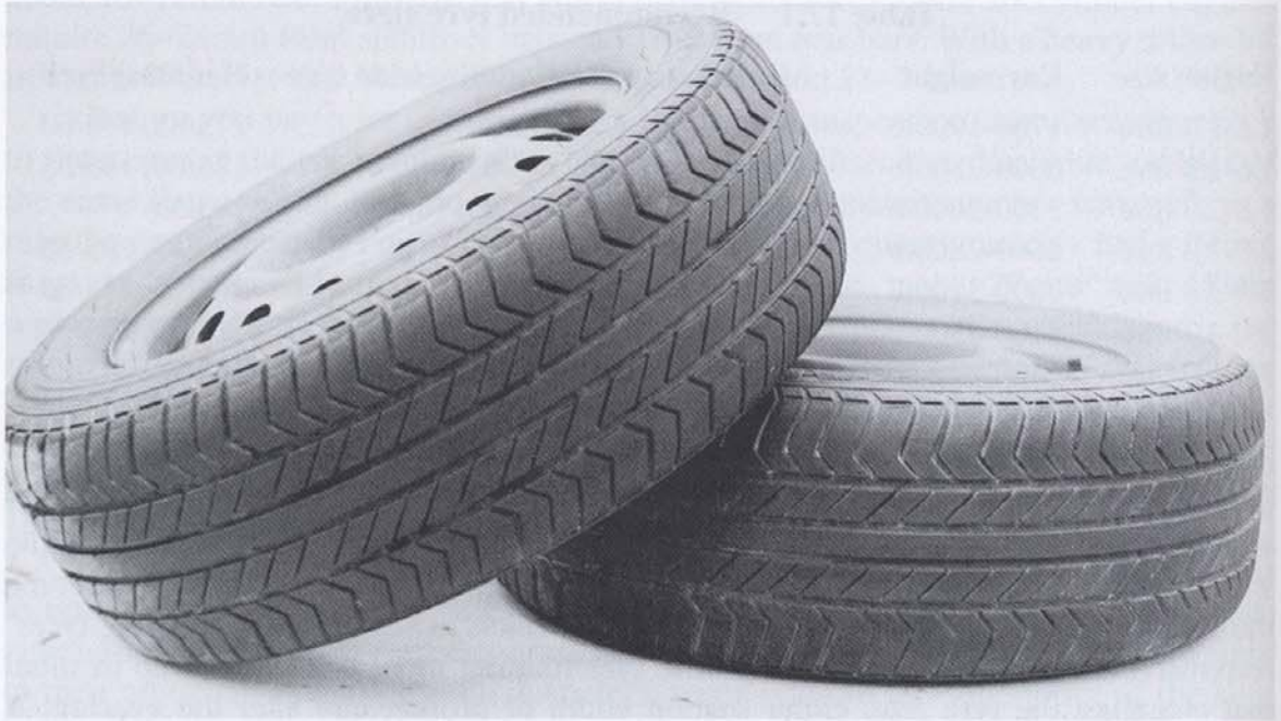
Michelin MXF Fizzarrows exhibit the sort of tread pattern to look for; good water channels running all the way around the tyre and drainage grooves to both the inner and outer edges from these channels.
