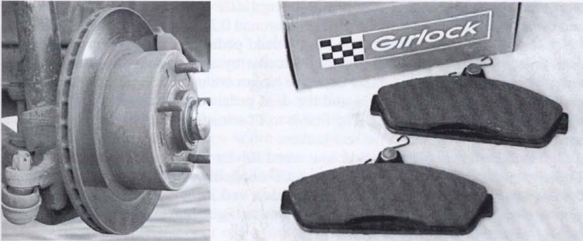
Ventilated discs at the front provide the needed braking performance when backed up by fade-resistant semi-metallic pads.
